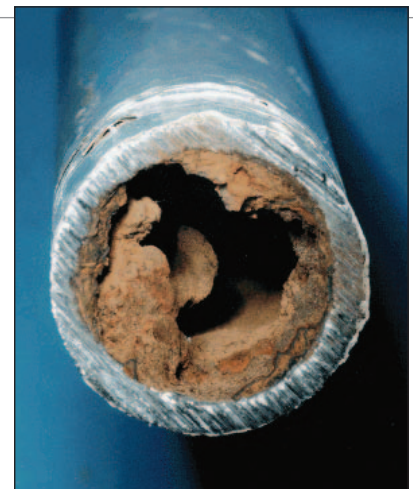
Durapipe ABS resists the limescale build-up common in most metal pipe materials as shown in the picture above.
