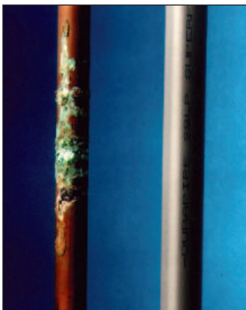
Durapipe ABS, unlike copper or steel, is free from corrosion.
